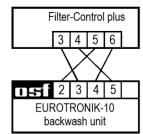
A 4-wire connection (12V Safety Extra Low Voltage) is required for connecting the EUROTRONIK-10. Ensure that the wires are connected to the correct terminal at each end. The EUROTRONIK-10 additionally requires a separate power supply. The backwash times are programmed on the EUROTRONIK-10.
